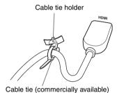
\* Use a cable tie of less than 1.9 mm × 3.8 mm thickness.
