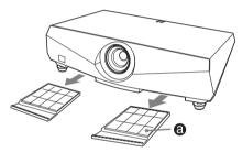
**3** Remove the air filter from the each claws (6 positions) on the air filter cover.
